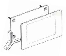
Attach the QR Code plaque: Use the alignment tool and transfer tape to precisely position and press the QR Code plaque onto the backplate. Apply consistent, firm pressure across the entire surface of the plaque for at least 30 seconds to ensure full contact and bond strength.
