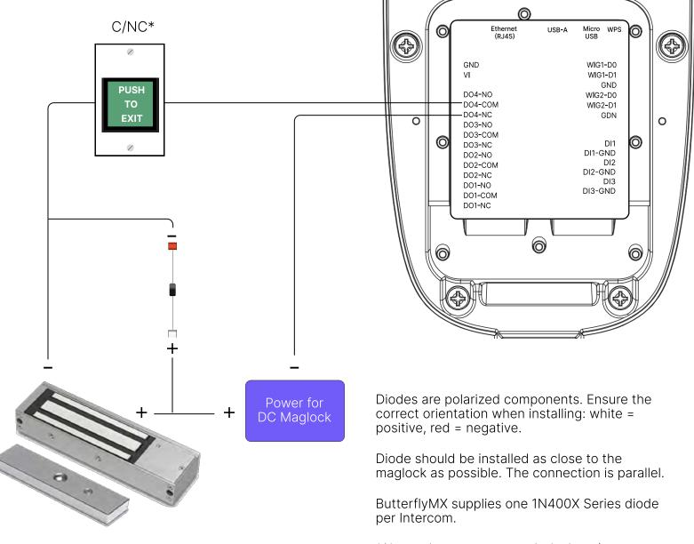
\*Alternative request-to-exit devices (e.g., motion sensor) can replace the Push to Exit button. They must be connected to C/NC. Any exit device must have a built-in timer.
