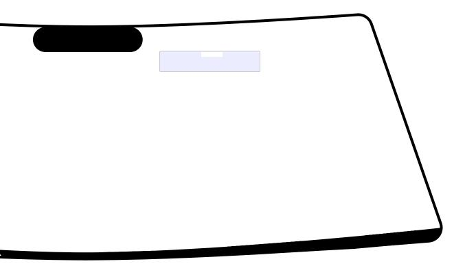
Athermic windshields impact the performance of the Vehicle Reader, as the metal on the windshield blocks the Reader from reading the Tag.
